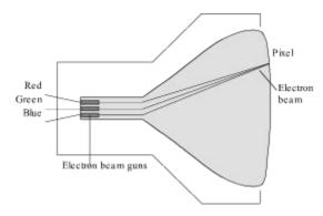
Switching the electron beam on and off creates a dot matrix which creates a monitor image. The individual dots are called pixels (=picture element). Each pixel has a red, a green, and a blue phosphor, a so-called triple. If all three phosphors are illuminated with equal intensity, the pixel appears white.
